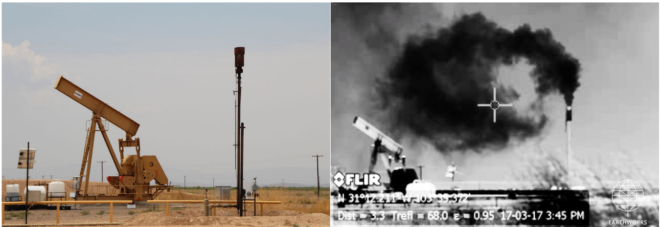
Left image shows normal view of West Texas oil and gas facilities. Right image is infrared view of the same facility, showing normally invisible pollution.
